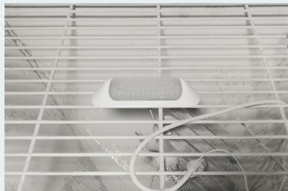
Fig.1-6 After IP6KX test
